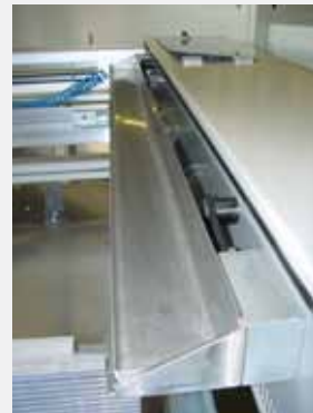
Pic. 14: Optional 90° squeegee swivel device ←
