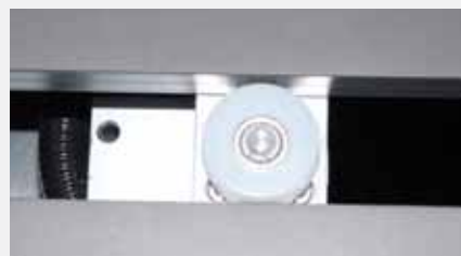
Pic.8: Centering roller in the print table
