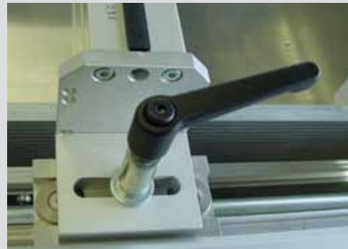
Pic. 13: Squeegee assembly set at an angle
