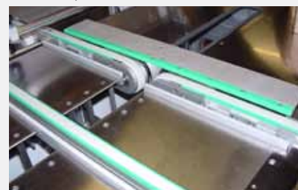
Pic. 4: Separated, outer conveyor belt with centering pusher
