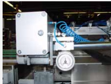
Pic.10: Micrometer spindle for micro-adjustment of the screen
