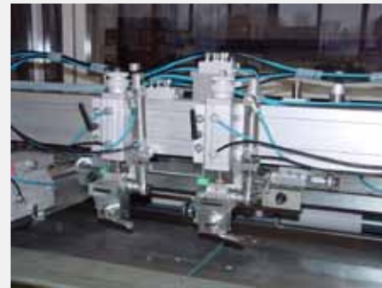
Pic.20: Anti-drip device with tilting cylinders
